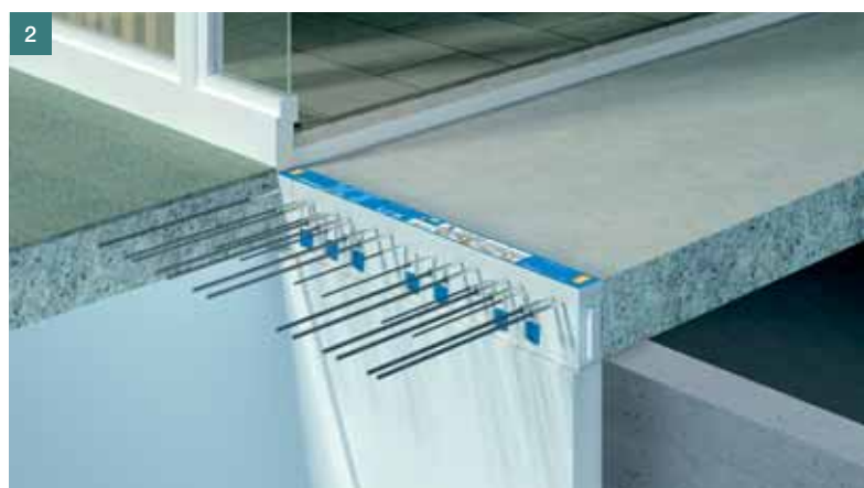
Fig. 2 Model of the built-in thermal insulating component Schöck Isokorb®
