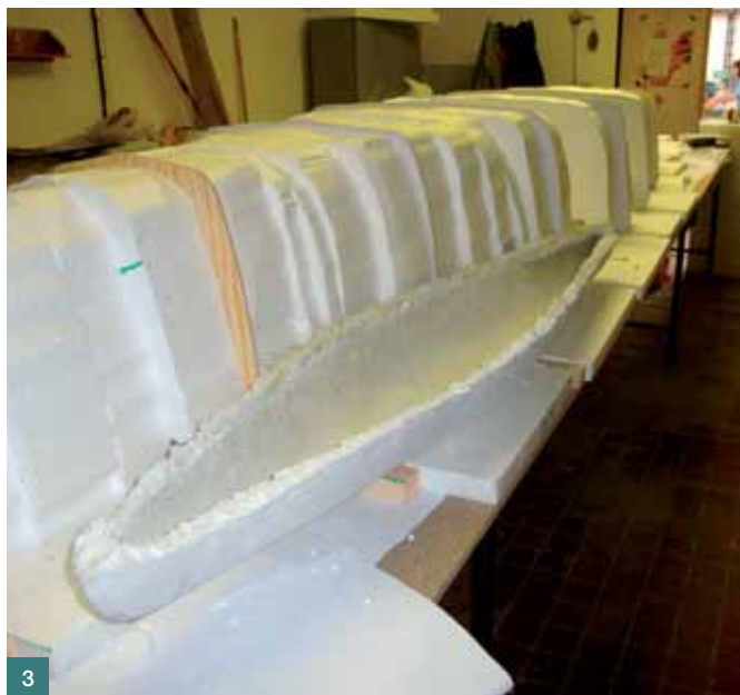
Obr. 3 Porovnání modelu s velkou formou ■ Fig. 3 Comparison of small scale model with final formwork
