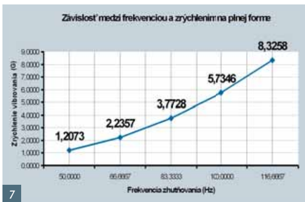
Fig. 8 Dependence between frequency and amplitude of vibration
