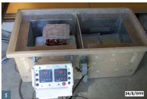
Fig. 5 Air-conditioner box T2000 without cover with specimens
