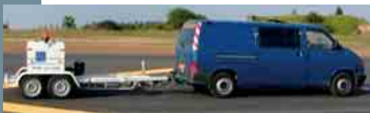
Fig. 2 Diagnostic equipment FWD CarlBro PRI 2100 suitable, among others, for measurement of load-bearing capacity of heavy concrete pavements
