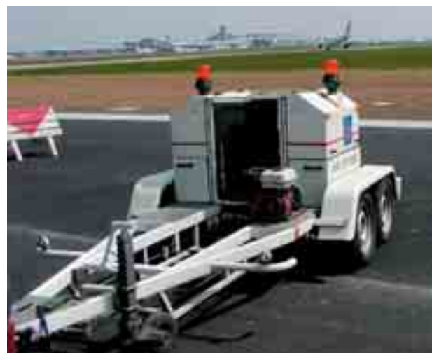
Fig. 3 View of CarlBro PRI 2100 equipment (measuring beam and loading mechanism) used in measurement of pavements at the Prague-Ruzyně airfield
