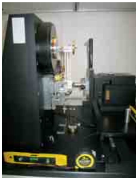
Obr. 2 Nanotest nanoindenter, Micro Materials, UK
