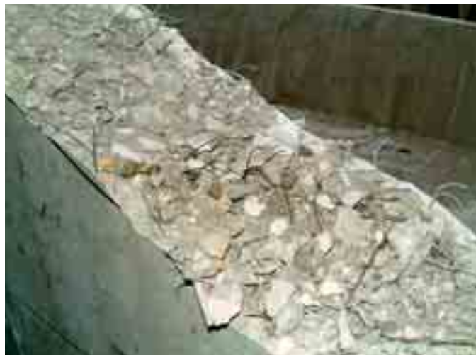
Fig. 7 Fracture surface of experimental girder
