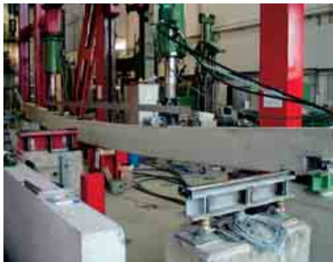
Fig. 9 Roof beams – load test in iBMB
