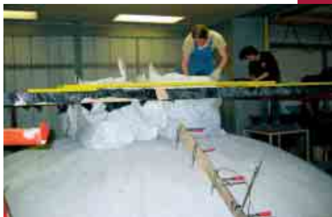
Fig. 6 Loads in the center-area of the shell, in the foreground: inductive deformation measurement devices
