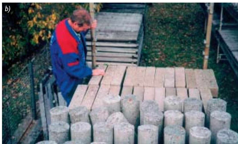
Fig. 1 a), b) Placement of samples of fly ash and reference concrete in the high-elevation lab
