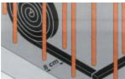
Fig. 7 Swelling butyl rubber strip put in the construction joint between the foundation plate and the wall
