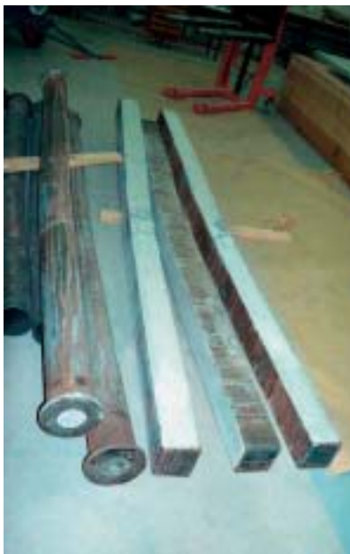
Fig. 8 Applied specimens TR Ø 152 x 4,5 and HE 140A, l = 3 m
