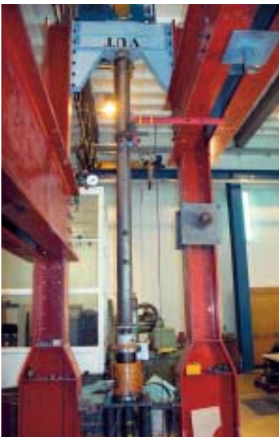
Fig. 7 Specimen TR Ø 152 x 4,5, l = 3 m test in compress
