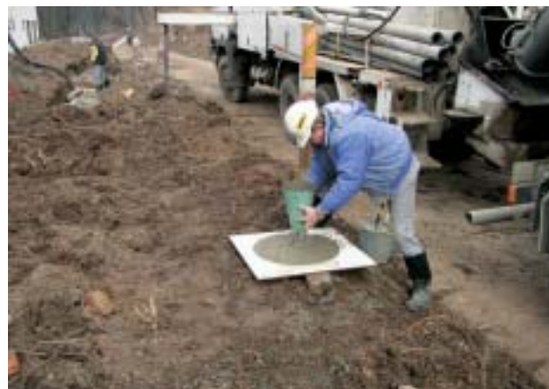
Obr. 7 Kolektor v Brně, stanovení konzistence metodou slum-flow test Fig. 7 Collector in Brno, consistency determination by the slum-flow test
