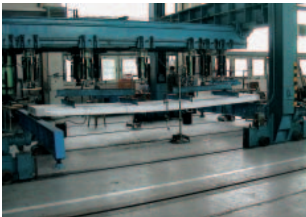
Fig. 1 Measurement of deformations of prestressed panel of Spiroll type, 7.2 m span; the loading test is performed within the certification of the product
