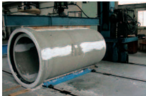
Fig. 2 Loading test (apex pressure test) of a reinforced concrete tube with the diameter of 1000 mm performed as part of the certification of the product
