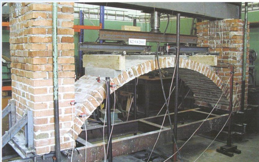
Fig. 1 Test of a clay brick arch
